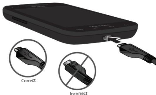
1. Plug the flat end of the Travel Charger into the Power/Accessory Interface connector and the other end into a standard AC wall outlet.
