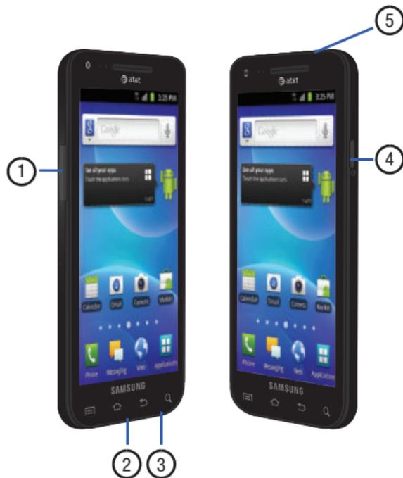
1. **Volume keys:** allow you to adjust the ringer volume while in standby mode or adjust the voice volume during a call. When receiving an incoming call, briefly press down either volume key (
