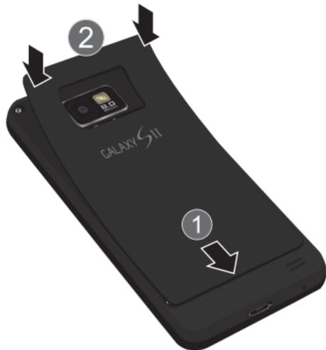
2. Press along the edge of the back cover (3) until you have a secure seal.
